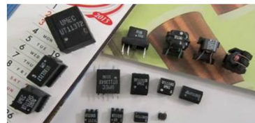
Data Coupling Transformers
