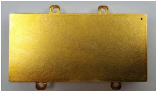
DC-DC converter 20V to 70V ,28Vo 112W
