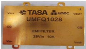
EMI Filter 0V to 70V , 10A
