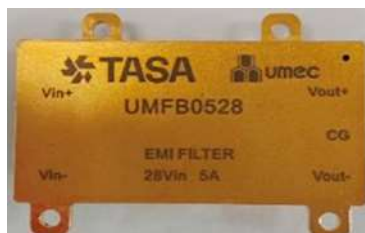
EMI Filter 0V to 70V , 5A
